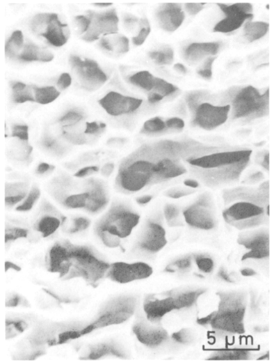
Figure 11 Typical example of fracture surface. Alloy 1 aged at 900^\circ\text{C} for 8 h.
